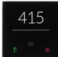
9025GL03P03 Door panel 2 ch. - Single glass - Black + RGB DND/MUR + Bell
